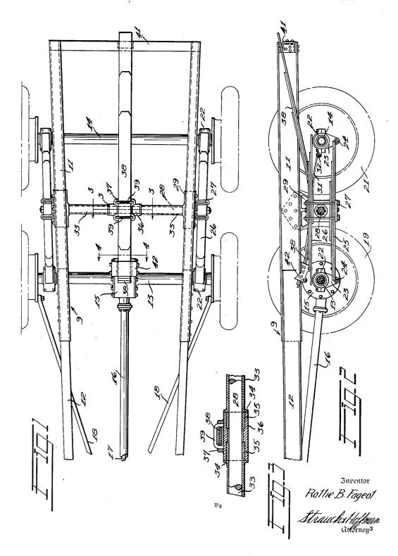
MULTIWHEEL VEHICLE OF THE TANDEM AXLE TYPE
